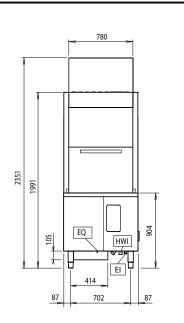
Drain ΕI Electrical inlet (power) EO **Electrical Outlet** HWI Hot water inlet
